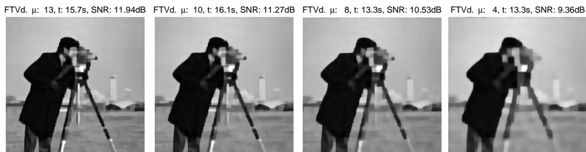
FIG. 4.3. Recovered from  $15 \times 15$  sized Gaussian blur with salt-and-pepper noise from 30% to 60% (left to right).
